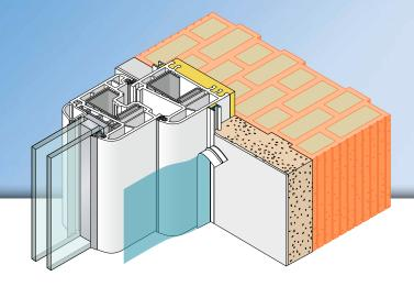
The **APU** window reveal bead MINI is used with indoor and outdoor plaster systems as specified by the latest APU selection criteria. Within the reveal the profile is stuck flush to the structural element there and thus forms a clean and reliable termination of the plaster.
