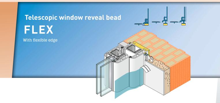
The **APU telescopic window reveal bead FLEX** is used indoor and outdoor plaster systems as specified by the latest APU selection criteria. Within the reveal the profile is stuck flush to the structural element there and after completion of the plastering work forms a clean and reliable termination of the plaster.
