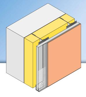
For back-ventilated rainscreens the **APU clip-on profile VHF-FIN-TEX** is used as a termination onto the edge of the supporting board.
