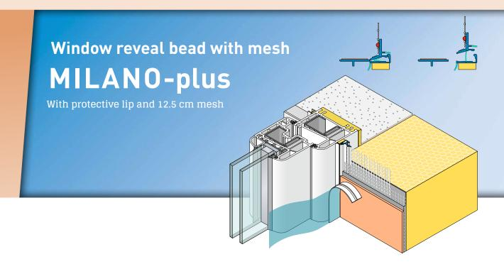
The APU window reveal bead with mesh MILA-NO-plus is used in compound heat insulation systems as specified in the latest APU selection criteria. Within the reveal the profile is stuck flush to the structural element there and after completion of the plastering work forms a clean and reliable termination of the plaster.
