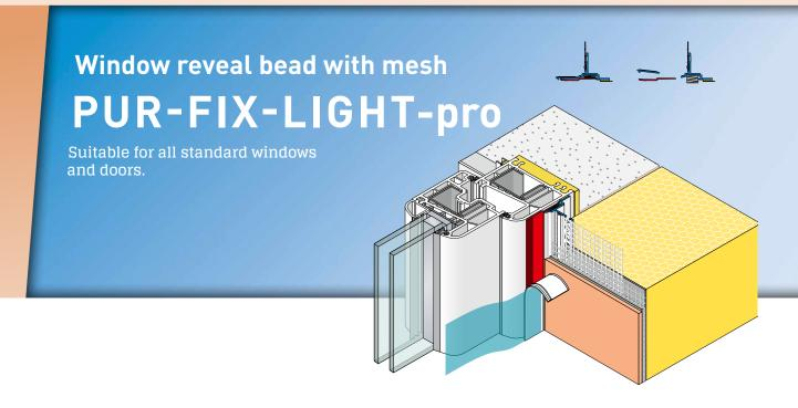
The APU window reveal bead with mesh PUR-FIX-LIGHT-pro is used in compound heat insulation systems as specified in the latest APU area of application. The profile is put in place shortly before the insulation of the reveal, is fixed flush to the structural element and after completion of the plastering work provides a clean and reliable termination of the plaster with a shadow gap.
