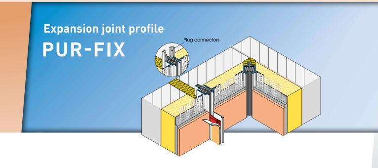
The APU expansion joint profile PUR-FIX is used in compound heat insulation systems at vertical building joints. For the flush formation of a clean plaster edge, the profile can be fitted both in flat surfaces and inner corners.
