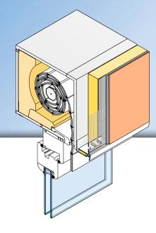
The **APU stick-on profile ZERO** is used horizontally in compound heat insulation systems e.g., for plaster joints up against shutter boxes.
