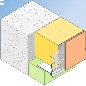
The **APU base edge profile SOKA-FIX-DUE** is used in compound heat insulation systems as the bottom termination of the wall insulation.
